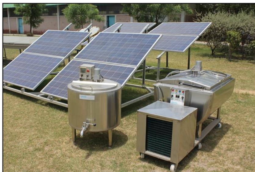
Figure 14.1 Newly developed solar-assisted milk chiller
